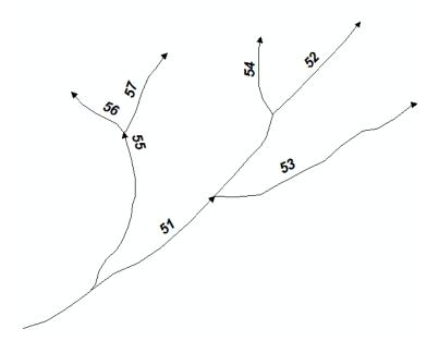
Use the *Create Routes* geoprocessing tool to create a measured line for each stream, based on the stream ID, with the measures starting in the lower left. Note that you can tell from the shape property whether a line theme contains measures (Polyline *M*)
