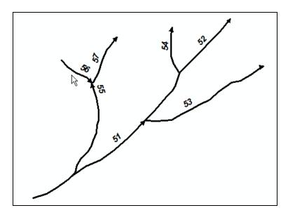
Use the *Flip Line* geoprocessing tool so all stream lines go upstream.
